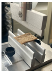
Figure 3. Texture Analyser with three-point bend rig
